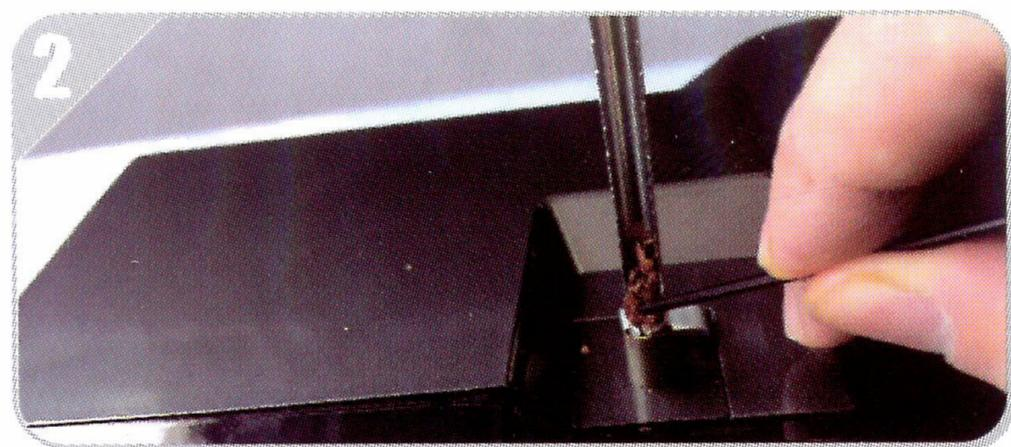
Use probe tool to remove tobacco left on the spoon. Scrape the back of the spoon, it must be completely clear of residue.
