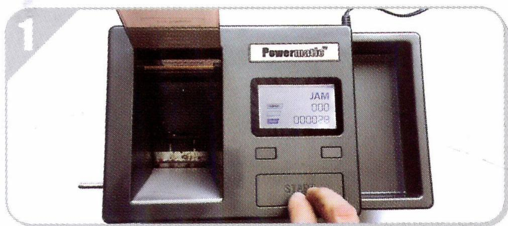
When JAM light is on, press the “START” button. Continuously press until the spoon is fully out.
