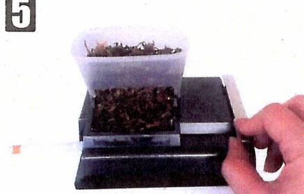
Press the handle down completely and then the paper tube will be filled automatically.
